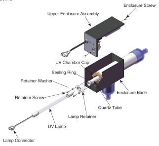
Figure 2: Spa Solar Eclipse Exploded View
