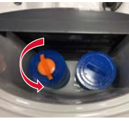
Turn Filters Counter-clockwise to Remove
