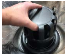
Pull Up to Remove Floater Assembly
