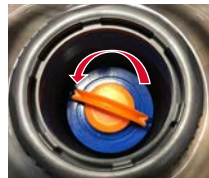
Turn Filters Counter-clockwise to Remove
