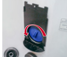
Turn Filters Counter-clockwise to Remove
