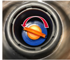
Turn Filters Counter-clockwise to Remove
